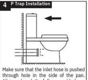
Align and push the fully assembled pan cistern back to the wall, connecting the pan spigot to the pan
