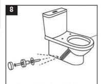
Fix the pan to the floor using the screws and caps provided. Silicone the pan to the floor and remove excess sealant.
