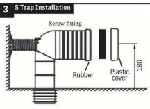
Lubricate the rubber fins of the pan bend and position this in the waste pipe at the correct height. Fix the pan
