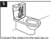
the wall using the appropriate plumbing fittings. Ensure the inlet valve filter (supplied) is installed onto the inlet valve. (Warranty will be voided if the filter is not installed). Fill the cistern the correct height.
