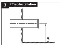
Set up the waste pipe to that the end of the pan collar extends 240mm from finished wall.
