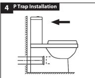
Make sure that the inlet hose is pushed through hole in the side of the pan. Align and push the fully assembled pan and cistern back to the wall, connecting the pan spigot to the pan collar. Bucket flush and check for leaks.
