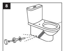
Fix the pan to the floor using the screws and caps provided. Silicone the pan to the floor and remove excess sealant.
