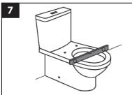
Ensure that the pan is level and that the cistern aligns with the wall. Make minor adjustments if necessary. (Note: walls may be out of square with floors which may create a gap behind the cistern. This can be covered up by using a suitable flexible gap filler.)
