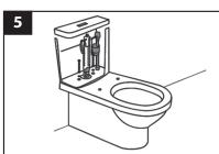
Connect the cistern to the stop tap on the wall using the appropriate plumbing fittings. Ensure the inlet valve filter (supplied) is installed onto the inlet valve. (Warranty will be voided if the filter is not installed.) Fill the cistern to the correct height.
