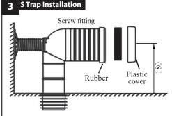
Lubricate the rubber fins of the pan bend and position this in the waste pipe at the correct height. Fix the pan connector back to the wall using the screw fitting and collar. (The screw fittings need to be cut down to size so that pan connector is fixed in the vertical position.)
