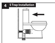
Align and push the fully assembled pan and cistern back to the wall, connecting the pan spigot into the pan connector. Bucket flush and check for leaks.
