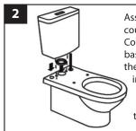
Assemble the cistern to the pan. Place the foam coupling seal into the pan recess (do not use sealant.)
