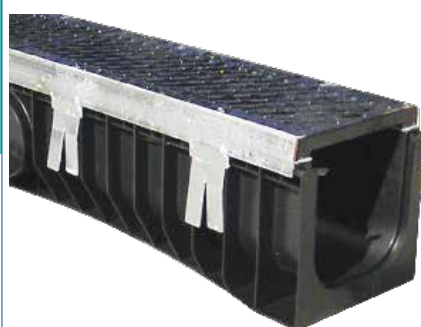
Technodrain Pro 150H HDPE Channel & Ductile Iron Grate (Class D) x 1m with 4mm Galvanised Edge
