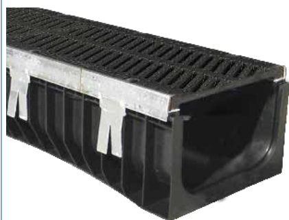
Technodrain Pro 200H HDPE Channel & Ductile Iron Grate (Class D) x 1m with 4mm Galvanised Edge
