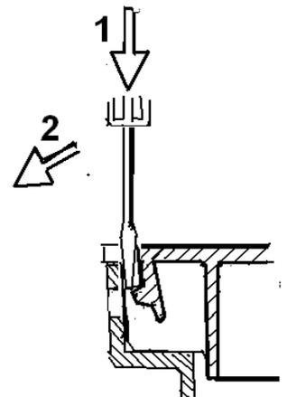
**Note** - Holes like those in the Box rim must be drilled in the Riser rim to allow the Cover to be locked.
