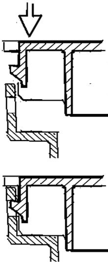
The Box Cover is positioned so that the two sides with moulded cut-outs are above the holes pre-drilled in the Distribution Box rim. The Cover is then simply pressed down until the locating pins moulded at the cut-outs engage with the drilled holes.
