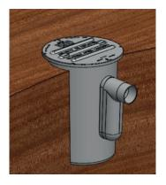
2. Remove the polymer grease trap lid. Pour a concrete pad approximately 550mm square and 50mm deep around the top of the 45L Grease Trap.
