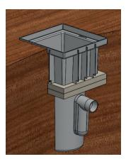
7. Install the Series 450 Polymer Lid on top of the riser. Insert stainless steel self tapping screws into the centre of the external sides of the polymer lid through the Series 450 Riser.
