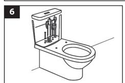
Connect the flexible water inlet hose to the stop tap in the wall. Fill the cistern and ensure correct water level. (A line inside of cistern indicates the correct water level.) The water level can be adjusted by using the screw fitting at the top of the float on the inlet valve.
