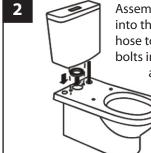
Assemble the cistern to the pan. Place the foam coupling seal into the pan recess (do not use sealant.) Connect the flexible hose to the inlet valve at the base of cistern. Position the fixing bolts into base of the cistern ensuring that the black washers
