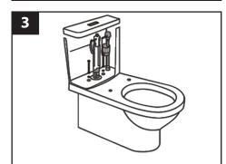
Feed the flexible hose through either the right or left hand hole in the pan. (Depending on the water inlet connection position.)
