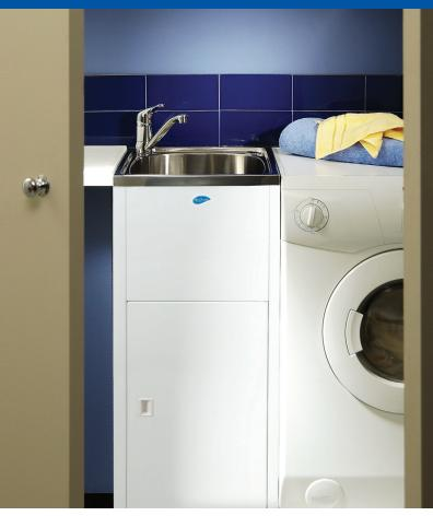
Code: 71196 Dimensions: 397mm wide x 570mm deep, 870mm high Cabinet: • White Powder Coated Galvanised Steel Cabinet • Left or right hand opening door • Two washing machine hose holes on each side of the cabinet with protective grommets and blanking plugs Floor Bowl: • Silk finish 304 Stainless Steel 30L Square Bowl • Two tap holes with single bypass Chrome basket waste (50mm) · Chrome plated blanking plug with nut
